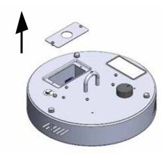
STEP 2: Attach raceway (flex metal conduit) and fittings to enclosure plate.
