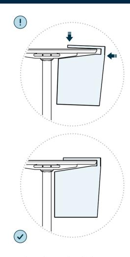
Remove the Hanging Desk Cubby from the box, and slide the top tray over the edge of the desk. Ensure that the Hanging Desk Cubby is flush to the desk's edge and level with the desk's top. Flip the Marker Board, which ships face-down, over before use.
