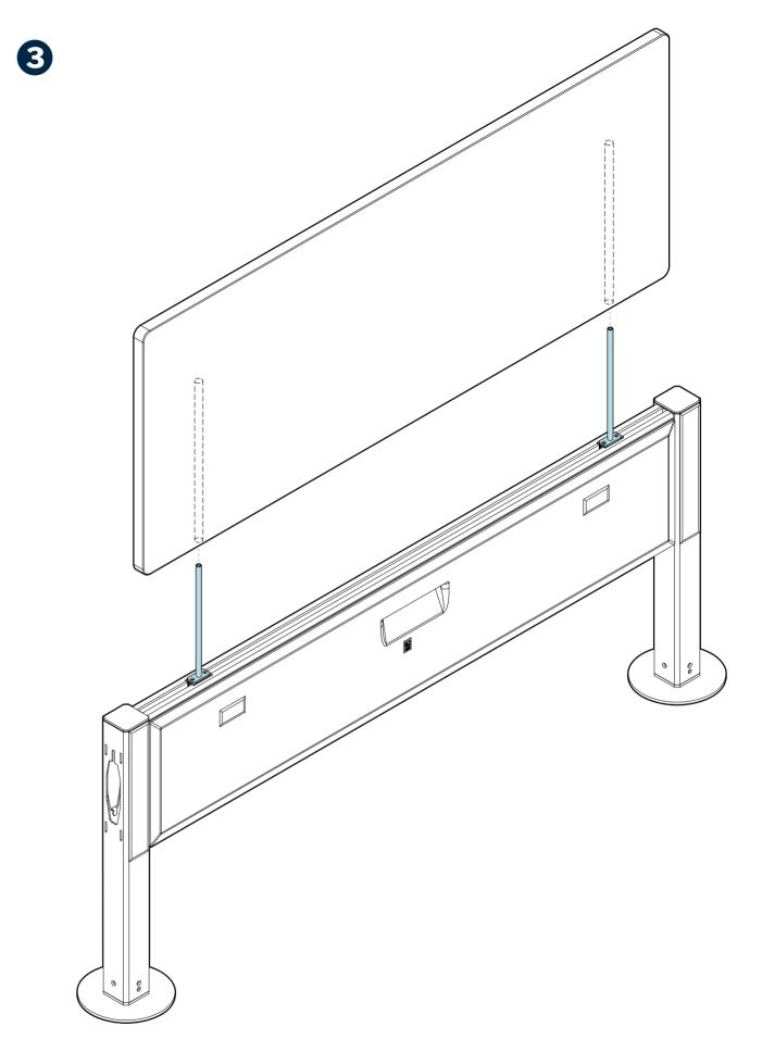
Position the panel with the predrilled holes facing down and aligned with the t-brackets, then lower the panel onto the t-brackets.
