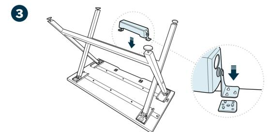
Find the cable management tray. Slide the tray into the notches above the bracket and push until it clicks, indicating it's locked into place.
