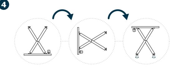
With one person on each side of the table, hold the legs and turn it on its side. Then turn the table into a fully upright position by holding the table top and turning it up onto its feet. Rotate the footpads to level the table as needed.
