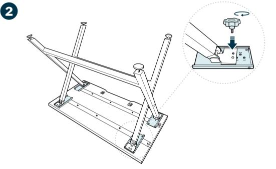
Table top and legs will arrive in separate boxes. Assemble the table with the table top face down in the box to prevent any surface scratching. Open the table top box and fold down all the cardboard box flaps. Remove the legs from their box. To ensure proper alignment, it's important to use the included cardboard guides to line up the legs at the track and slide the leg joints over the connection points. The table can be adjusted to one of seven heights.
